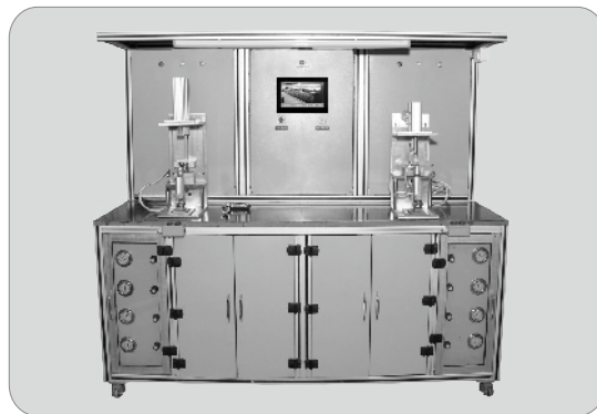
Air & Water Leakage Test
